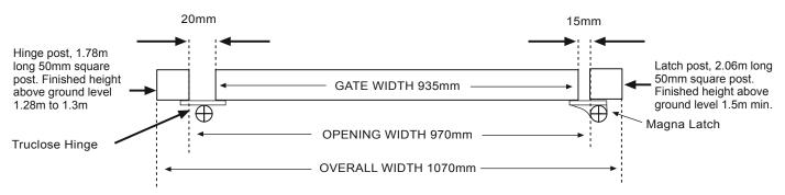
Remember the gate is to open away from the pool. Decide which side to concrete or bolt down the hinge and latch posts.
